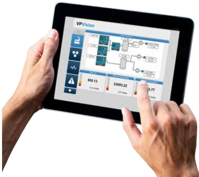
to take factual and well-founded decisions on your costs and investments. Reveal the consumption of all utilities, including compressed air, technical gases, steam, vacuum, natural gas, electricity, waste water, heating fuels etc. VPPVision enables you to view data on any platform from a PC to a smartphone enabling your organization to raise the energy awareness among staff and management. It will be your guiding hand for individuals, teams or at company-wide level to target energy savings.
